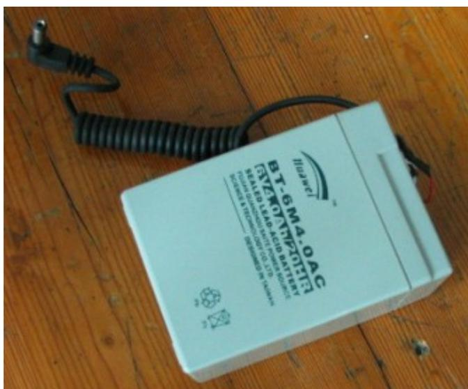
6V/4Ah Lead-Acid battery
